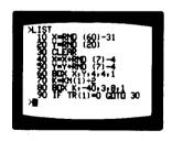
In Line 70, the variable K is set to the value of the knob KN(1) + 2. Line 80 draws a black box that is three squares wide and eight squares tall. The box can be moved left or right as the value of K changes. The center of the box can be moved left or right as the value of K changes. The center of the box will be at - 40, near the bottom of your screen.
